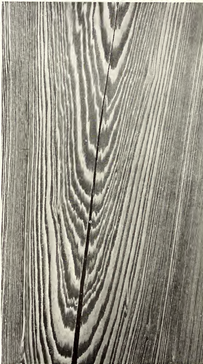
FIGURE 2-91.—Artificial spiral grain as indicated by oblique alignment of apexes of annual rings on the tangential surface (when diagonal grain is present). Natural spiral grain absent, as indicated by parallelism of split with alignment of apexes of annual rings.
